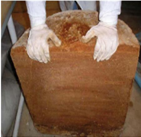
FIGURE 10: Cross-section of a 55 gal drum scale surrogate salt waste form produced by P. R. Mayak in Russia with funding from USDOE and in collaboration with Argonne National Laboratory (2007) (source: Argonne file photo).
