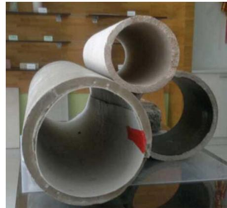
FIGURE 12: Demonstration of sewage pipe coating with Grancrete (Grancrete, Inc., Taipei, Taiwan) (<http://www.dynamo.com.tw>).
